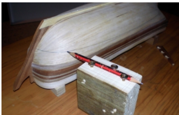
13. Hull supported so the base of the keel is parallel to the table top. Water level is marked on hull.
