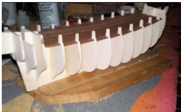
2. Plywood deck glued to secure the frames while beveling the edges.
